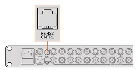
The RS-422 serial port lets you control Blackmagic MultiView 16 from third party routers and automation systems. The connector is an RJ11 connector, the same used in many landline telephone connections. By modifying an RS-422 to USB adapter cable terminated with an RJ11 connector, you can control Blackmagic MultiView 16 using external controllers via USB.
