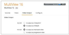
The radio buttons in the 'video output' tab for MultiView 16 are used to set the view layout, Ultra HD video format, HD output and SD aspect ratio
