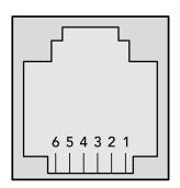
Pinout diagram for the RJ11 connector
