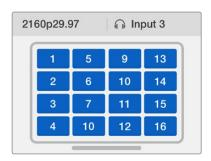
The 'home' screen is the default display on Blackmagic MultiView 16's control panel LCD. This screen displays your selected multi view layout, the frame rate for the multi view SDI output, and the selected SDI input used to embed audio into the multi view output.
