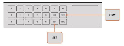
To set a source to a view, press the 'view' button to enter the view setting, make your selection, then press the 'set' button to confirm your setting
