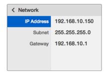
Use the rotary knob or the "1" and "2" buttons on Teranex Mini Smart Panel to assign values to your Blackmagic MultiView 4 network settings
