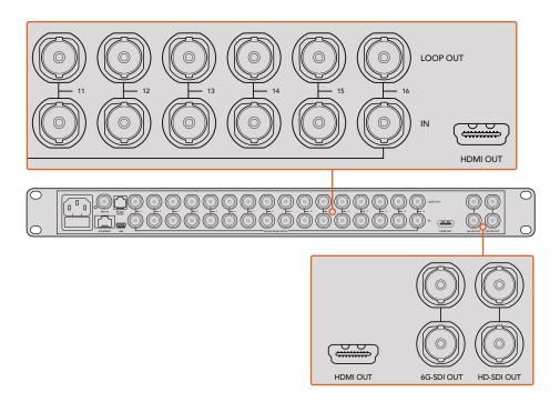
TIP All of Blackmagic MultiView 16's SDI and HDMI outputs can be used simultaneously for Ultra HD and HD multi view monitoring. On Blackmagic MultiView 4, you can select between Ultra HD or HD multi view output settings using the built in switches, an optional Teranex Mini Smart Panel, or via the Blackmagic MultiView Setup utility software.
