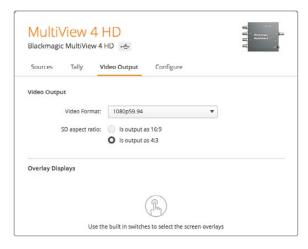
The'video output' tab for Blackmagic MultiView 4 HD lets you set the output  $\ensuremath{\mathsf{HD}}$  resolution and frame rate, plus set it to interlaced or progressive scan
