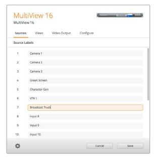
Use Blackmagic MultiView Setup to customize input labels so you can quickly identify each source within the multi view layout
