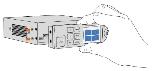
When installing the Teranex Mini Smart Panel to your Blackmagic MultiView 4, holding the panel with your fingers and thumb aligned with the panel's rear connector will help guide it into place
